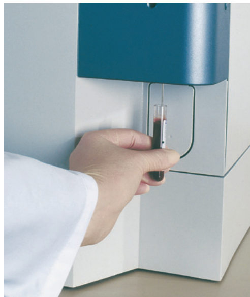
Fig. 4 In the XS-800i, blood samples can only be analysed manually and in open condition which is advantageous especially for minimal blood volumes.
