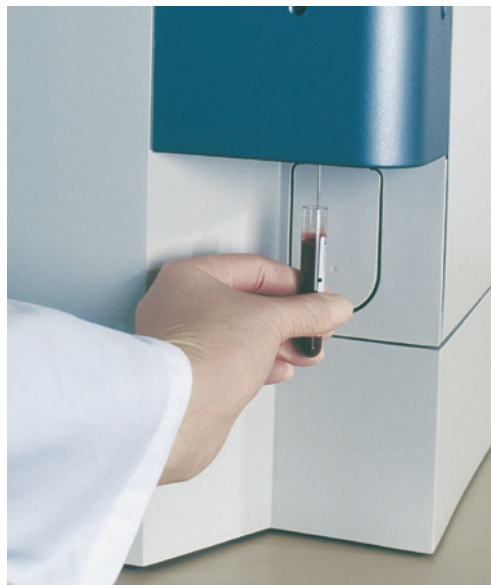
Fig. 4 In the XS-800i, blood samples can only be analysed manually and in open condition which is advantageous especially for minimal blood volumes.
