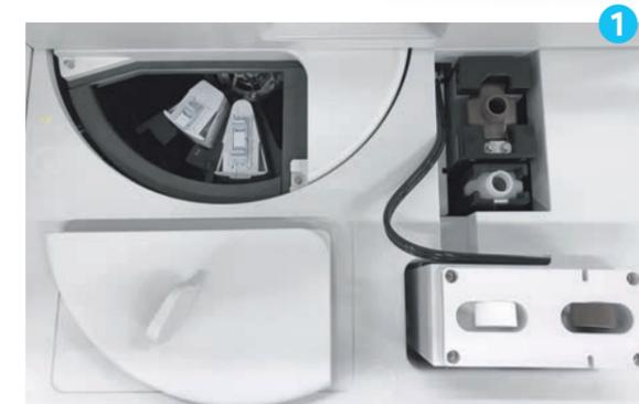
You can install up to five sets of reagents. Reagent information is managed by the barcode on the reagent bottle. Automatic opening and closing of reagent bottle caps prevent reagent deterioration, and the reagents are automatically agitated on a regular basis.
