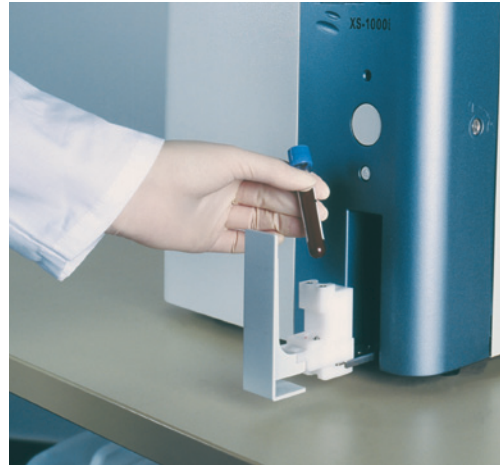
Fig. 9 XS-1000i: Closed sample position for piercing tube caps.
