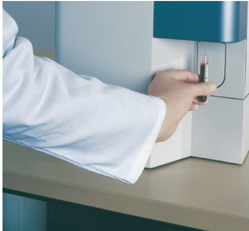
Fig. 8 XS-500i and XS-800i: Only 20 \mu L of blood are enough for 24 parameters, which perfectly fits the requirements of paediatric samples.
